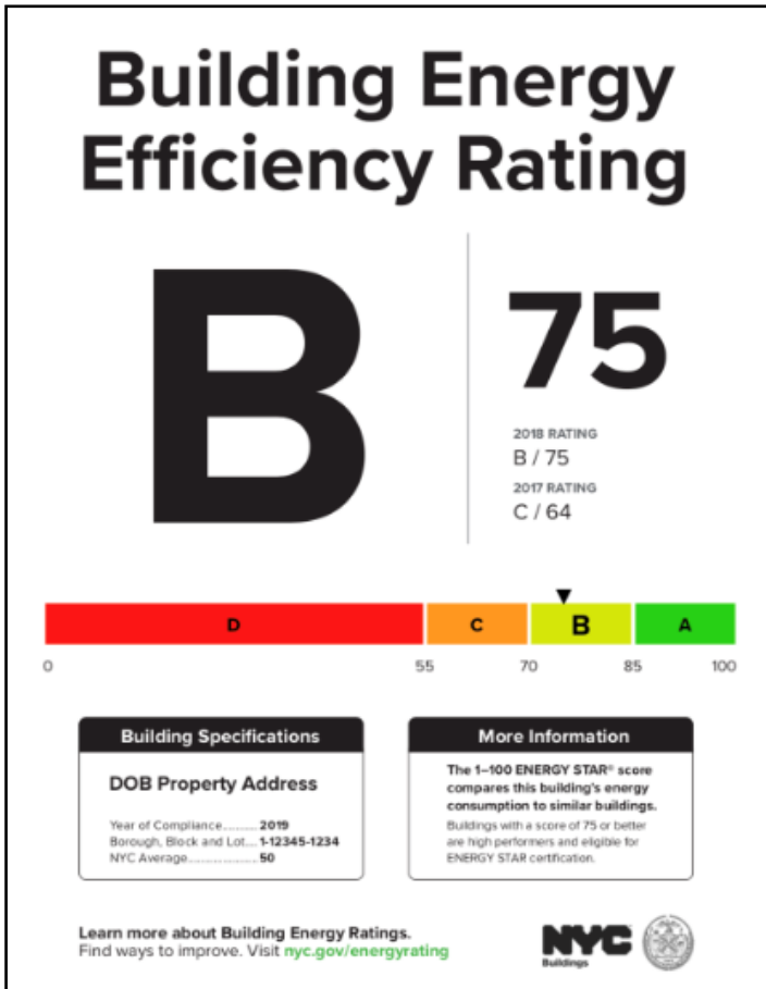
Sample energy efficiency label Grade to be posted in the building in compliance of Local Law 133
